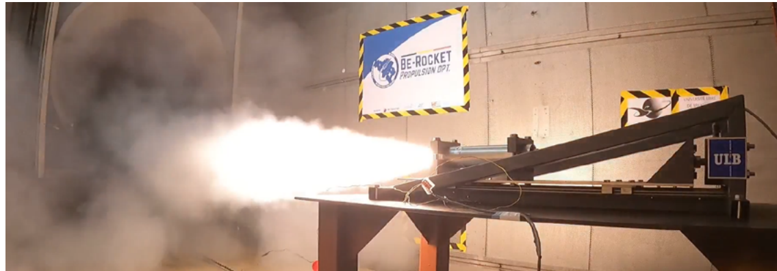
Test fire of our COTS rocket motor of the Bossart-I at Beauvechain air base
