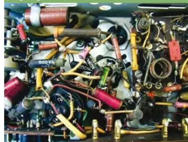
Radio wave receiver from 1948 before printed circuit boards (image: Eigelsreiter)
