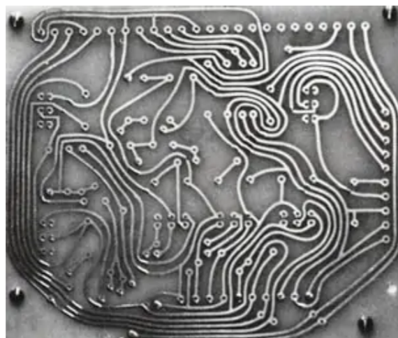
Printed circuit board from the year 1943 (Image: Kluger)
